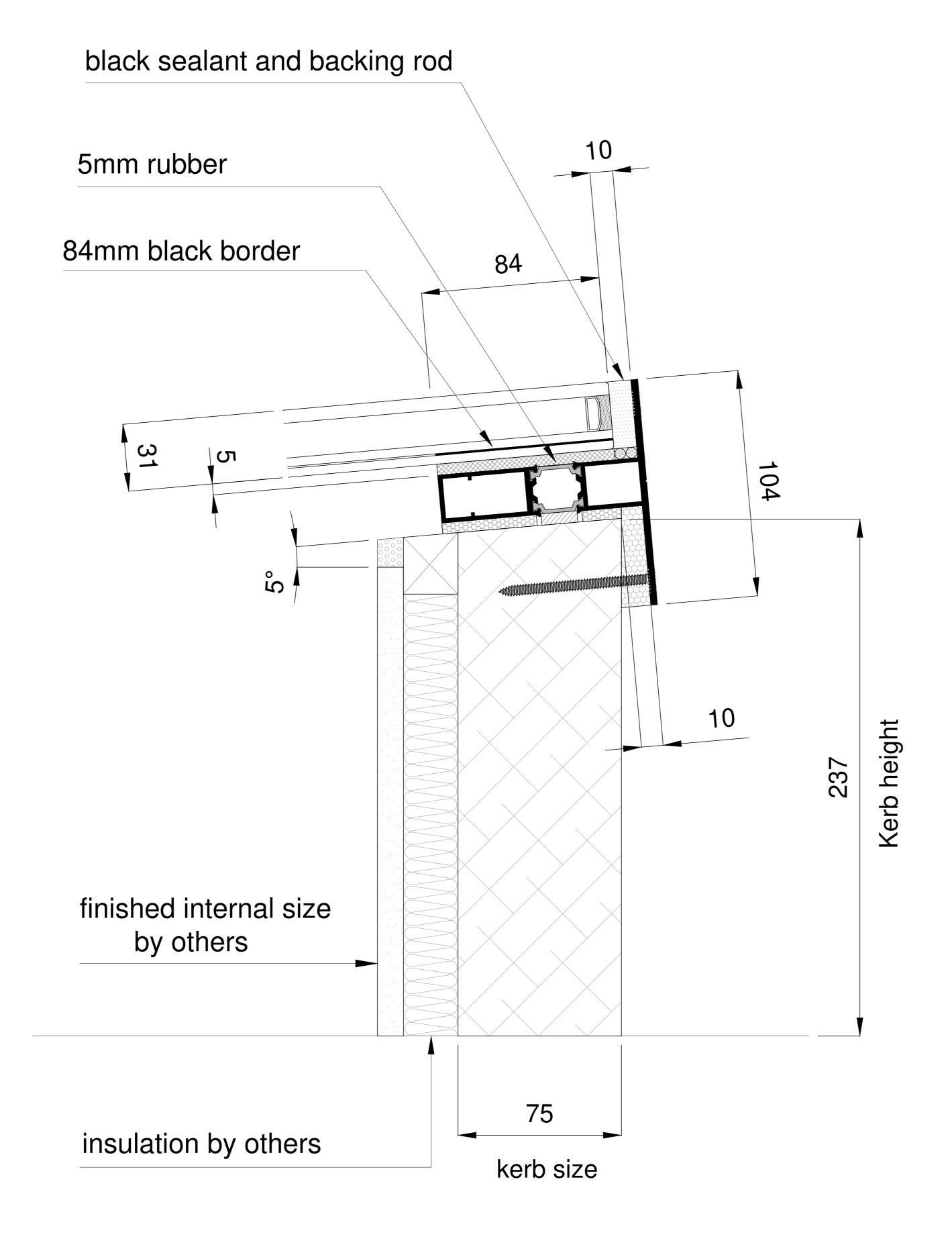
NOTE: STANDARD ROOFLIGHT External weathered kerb size 1000mm x 2000mm is a critical dimnsion to ensure the rooflight fits over the outside kerb
